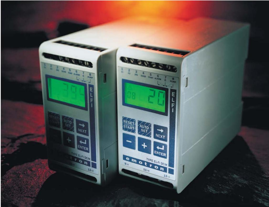
As the unit continuously monitors the pump running time, the period elapsed is used to determine the time of the following pause period. The longer the run period; the shorter the pause period. Thus pump operation varies automatically according to the pit filling rate.
