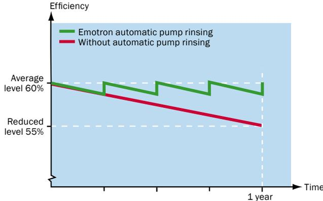
Emotron VSC offers automatic pump rinsing. In this example, a centrifugal pump at a sewage treatment plant is set to run at full speed for certain intervals to rinse out sludge, thereby increasing efficiency.
