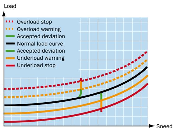
Emotron VSA protects your process against damage and inefficiency by sending a warning or stopping the process at your chosen load levels.
