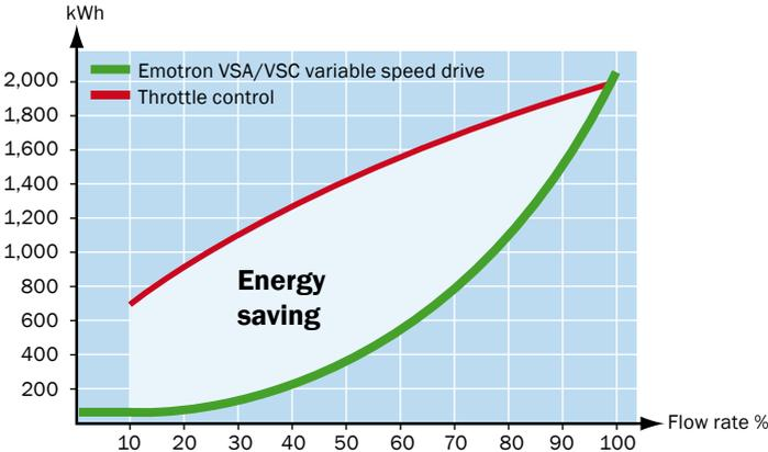
Speed control offers considerable energy savings. In this pump application, energy consumption is reduced by up to 50% compared to throttling valves. Calculation is made using Emotron Energy Saving Calculator and assumes a 2.2 kW motor.
