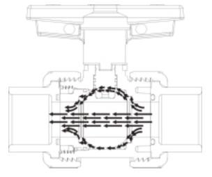
Since the seat is allowed to "float" in the open position, fluids and debris do not accumulate around and behind the seat. The result is a self-adjusting seat with reduced wear, smoother operation, and self cleaning action to keep the valve free of internal sediment and fluid stagnation.
